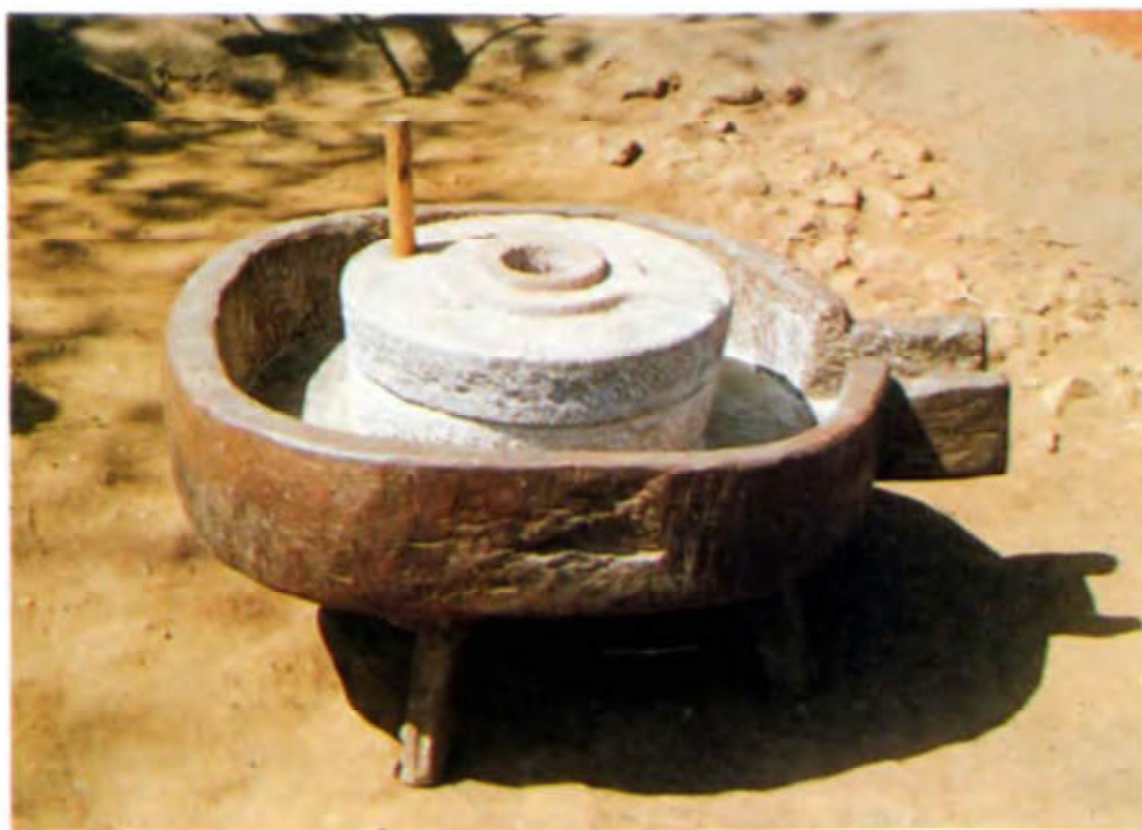
'Jatya' - A grinder with flour gatherer at bottom and handle of grinder, made from the wood of Tectona grandis .
