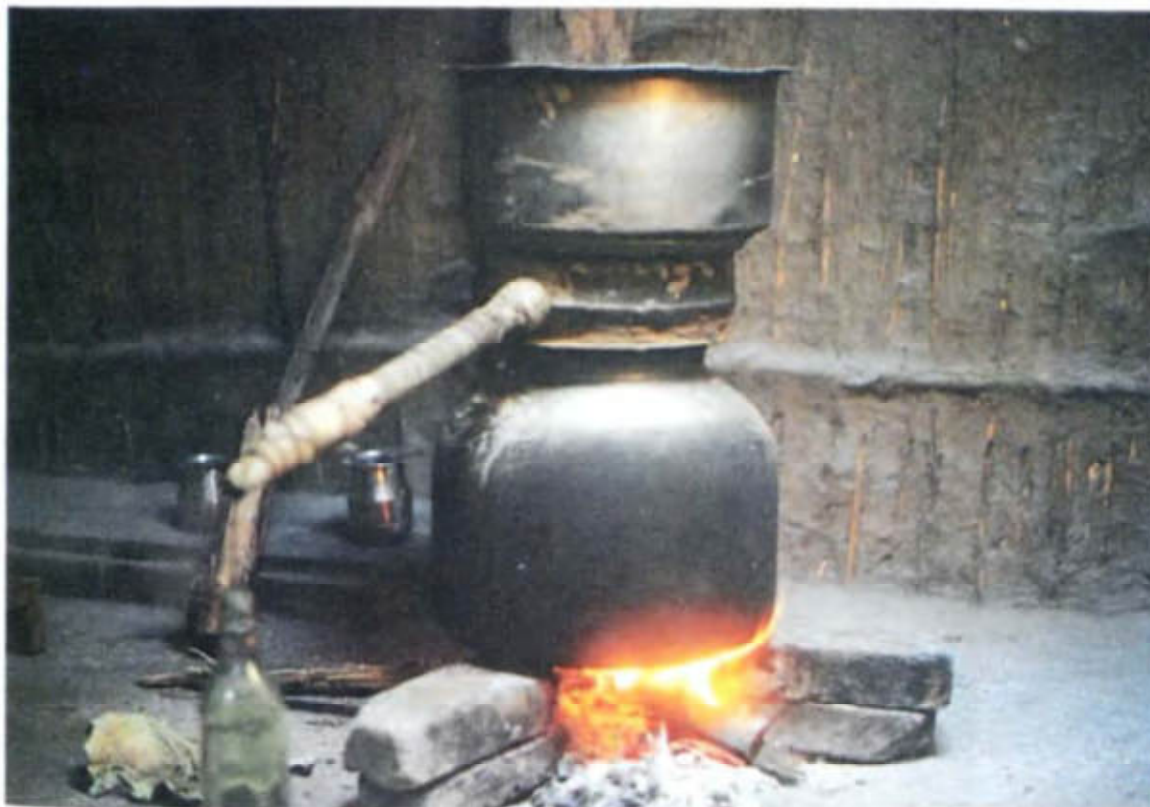
An apparatus set up for distillation of liquor from flowers of Madhuca longifolia var. latifolia .
